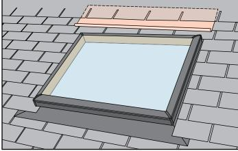
Take precautions on roofs where sliding snow and extreme water run off is likely to occur by installing a snow deflector or rain diverter (supplied by others) above any Thermo-Lite skylight with a frame width greater than 45". Thermo-Lite skylights with frame widths less than 45" may also require the installation of snow deflectors or rain diverters on roofs where there are hazards of sliding snow or heavy run off of water above the skylights.
