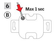
Press briefly the SET button on the back with a pointed object to register the new product. You can now operate the chosen product with (B).
