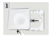
Press with a pointed object at the bottom of the holder and remove the back section.
