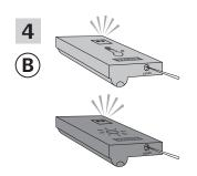
Prepare sensors for registration: Press the button at the bottom of the sensor with a pointed object for at least 5 seconds until the diode flashes.
