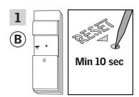
Press the RESET button on the back with a pointed object for at least 10 seconds to prepare the products for registration.
