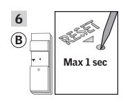
Press briefly the RESET button on the back with a pointed object to register the new product.
