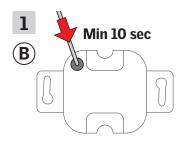
Press the SET button on the back with a pointed object for at least 10 seconds to prepare the products for registration.
