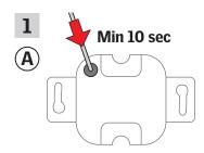
Press the SET button on the back with a pointed object for at least 10 seconds to prepare the products for copying.
