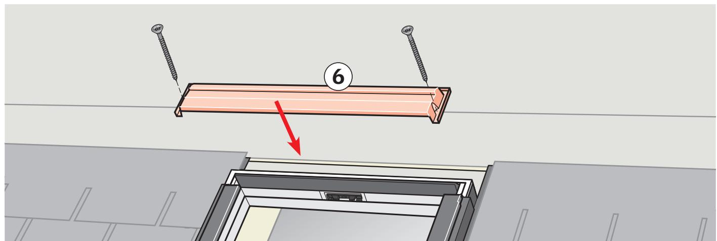
**ENGLISH:** Install and secure the top casing as shown.
