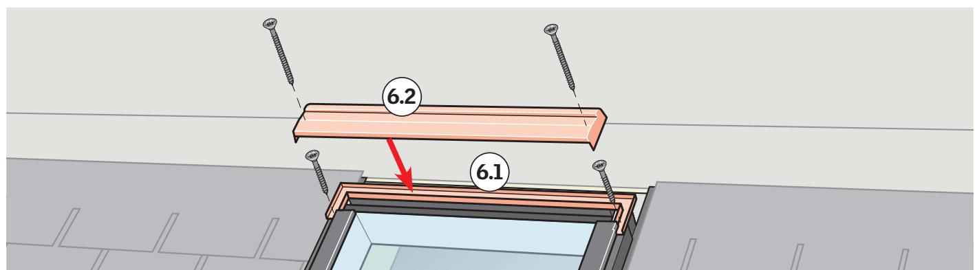
**ENGLISH:** Install and secure the two top frame cladding parts as shown.
