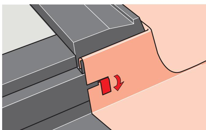
**ENGLISH:** Engage cladding with the saddle flashing and secure by bending flaps as shown.
