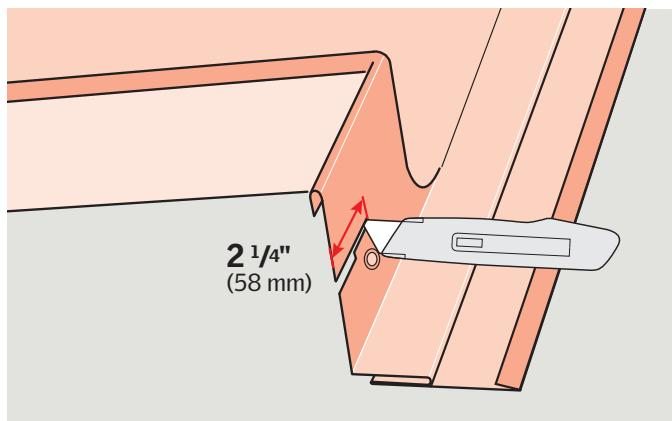
**ENGLISH:** Cut and extend the existing slit in saddle flashing section to depth as shown ( $2\frac{1}{4}$ " (58 mm)).
