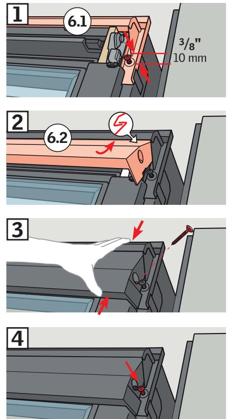
**ENGLISH:** Install and secure the two top frame cladding parts as shown.
