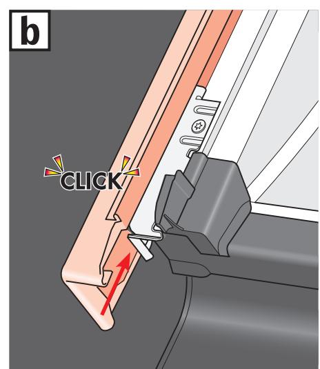
**ENGLISH:** Follow the instructions supplied with the flashing when installing the flashing at the sides. Install cladding as shown (a, b).
