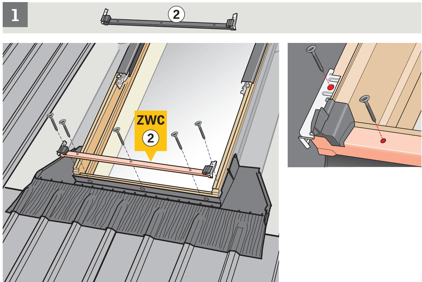
**ENGLISH:** Position sill flashing section tightly to the bottom frame. Install bottom frame cladding and secure with screws as shown.
