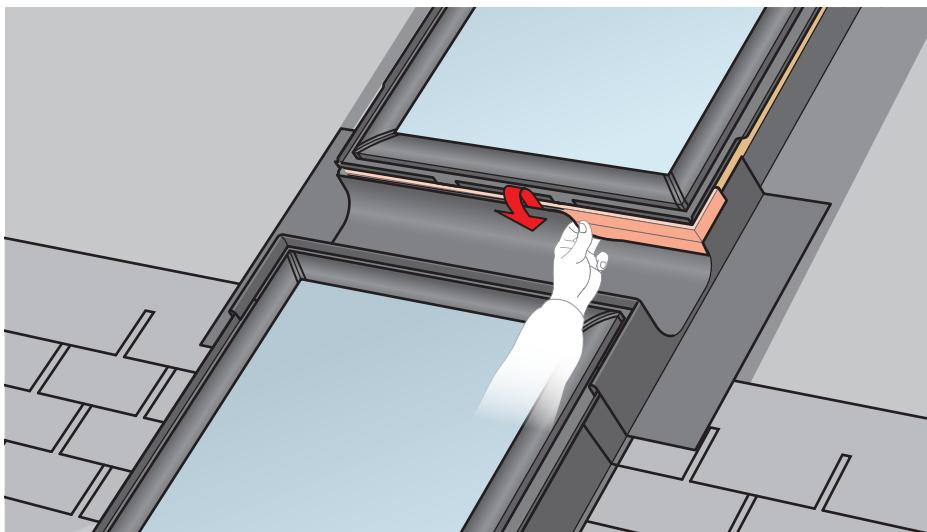
**ENGLISH:** Carefully lift up the bottom gasket of skylight FS and place it over the middle flashing section to allow for drainage into the middle gutter.
