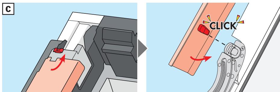
**ENGLISH:** Remove cladding parts as shown. Install cladding parts as shown (a, b). Replace cladding parts.
