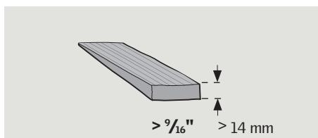
**ENGLISH:** EKL cannot be used for cedar shakes and slates thicker than 9/16" (14 mm). In this case, see installation instructions for flashing EKW (for profiled roofing materials).
