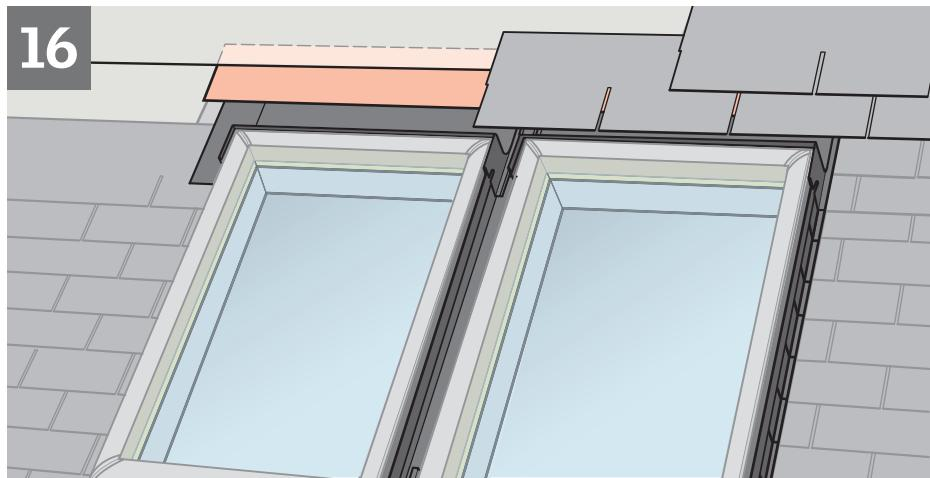
**ENGLISH:** To allow for proper drainage, interweave roofing underlayment as shown in **16a** for new construction applications. For retrofit applications, interweave roofing underlayment as shown in **16b**.
