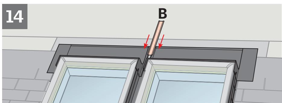
**ENGLISH:** Interlock saddle flashings using the long 16" (405 mm) slide strip (**B**) and flatten with hammer to lock.
