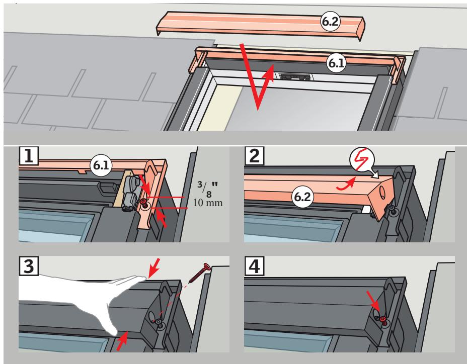
**ENGLISH:** Install and secure the two top frame cladding parts as shown. Make sure the cladding parts engage correctly (1, 2, 3, 4).
