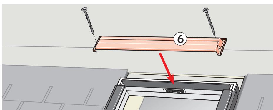
**ENGLISH:** Install and secure the top casing as shown.
