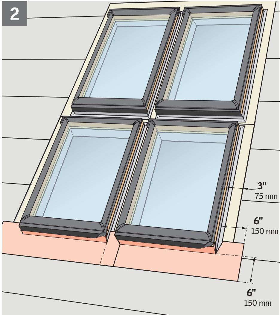
**ENGLISH:** To ensure waterproofing, skylight/roof window frames must be completely wrapped in VELUX adhesive skylight underlayment supplied with the flashing. This underlayment must be applied before installing the flashing.
