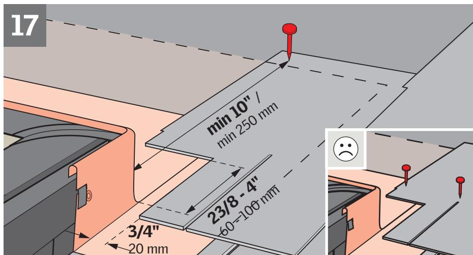
**ENGLISH:** Observe distance to roofing material. Do not nail through the saddle flashing when attaching the roofing material.
