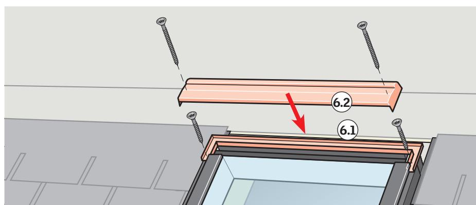
**ENGLISH:** Install and secure the two top frame cladding parts as shown.
