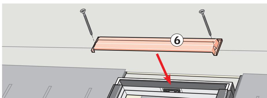
**ENGLISH:** Install and secure the top casing as shown.
