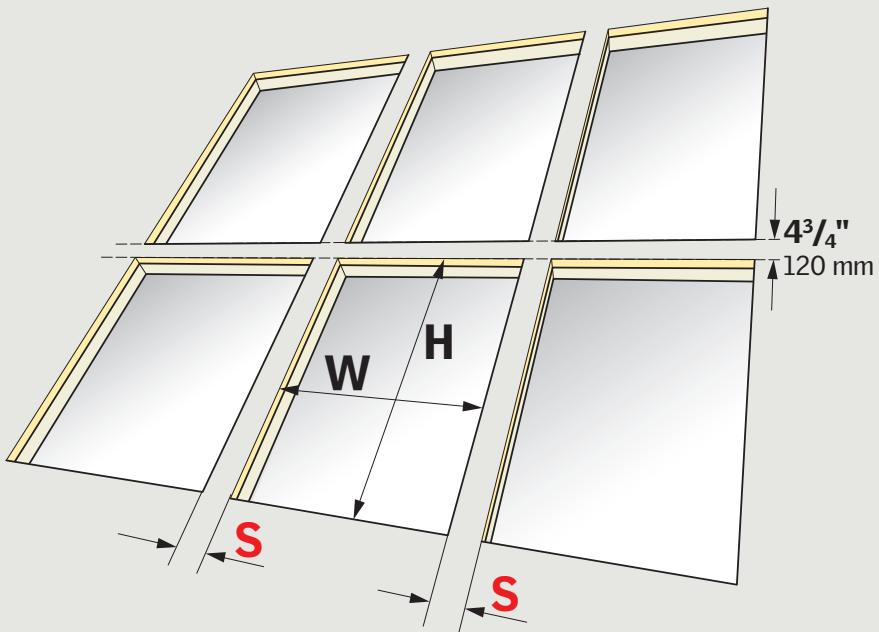
**ENGLISH:** Prepare rough openings with spacings and dimensions as shown. Use spacing **S** that corresponds to **a** (nominal frame spacing). Frame spacing **a** is specified on the EKL ---8 gutter.
