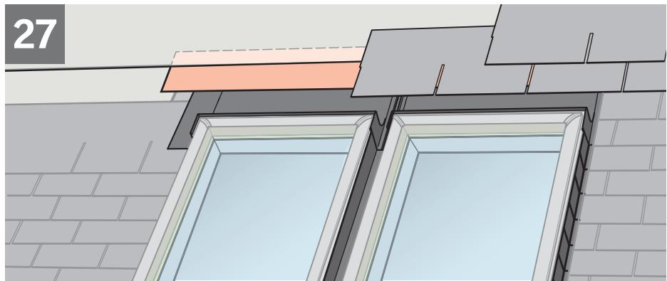
**ENGLISH:** To allow for proper drainage, interweave roofing underlayment as shown in **27a** for new construction applications. For retrofit applications, interweave roofing underlayment as shown in **27b**.
