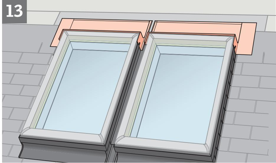
**ENGLISH:** Install saddle flashings. Determine use of extension piece: use it if the saddle flashings are lifted up by the underlying roofing material and remove it if the saddle flashings fit tightly over the skylights/roof windows.
