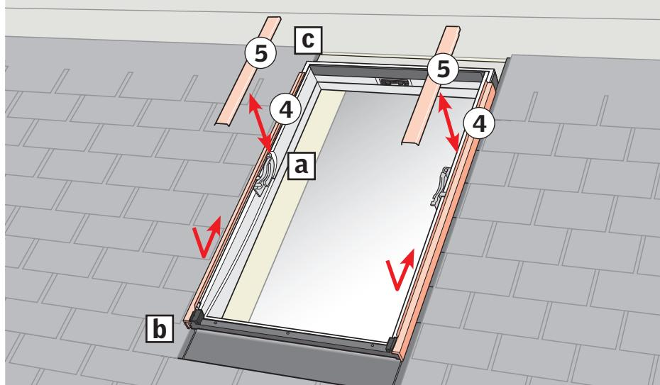
**ENGLISH:** Remove cladding parts shown (a). Install and engage cladding parts as shown (b, c).
