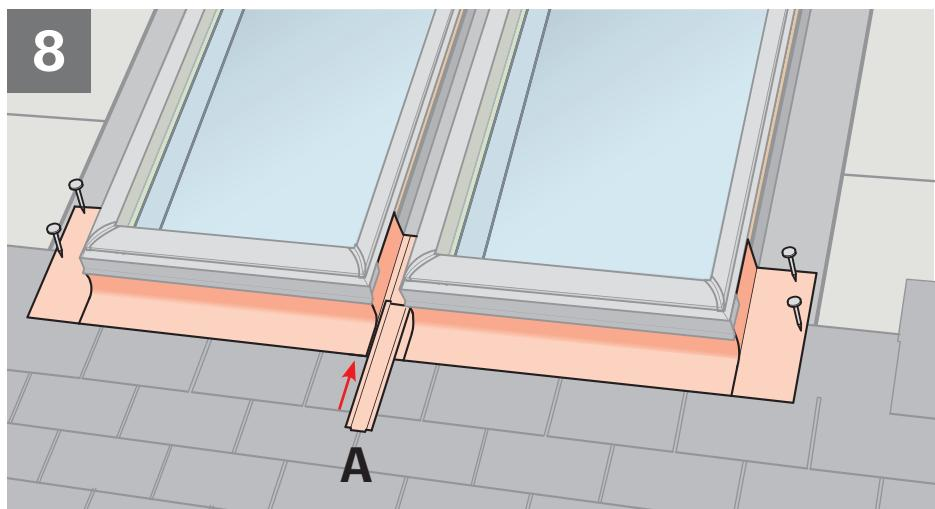
**ENGLISH:** Assemble sill flashing sections using the short 13" (330 mm) slide strip (**A**) and flatten with hammer to lock. Position sill flashing sections tightly to the bottom frames and attach them with roofing nails as shown.
