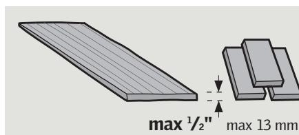
**ENGLISH:** EKL can also be used for cedar shingles and slates (max thickness 1/2" (13 mm)). In this case, download specific installation instructions for flashing EKL for roofing material cedar shingles and slates or contact your VELUX sales company.
