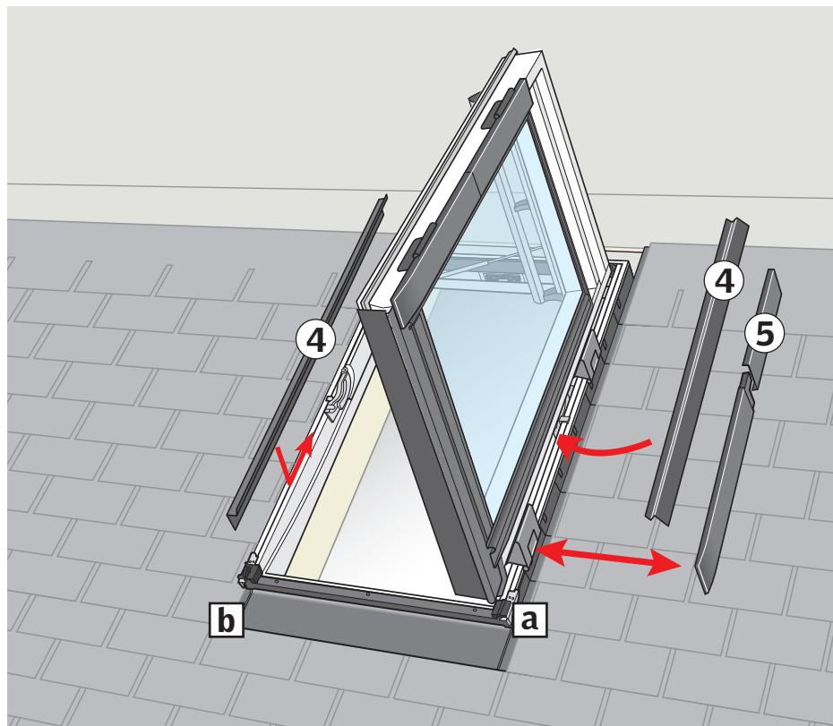
**ENGLISH:** Remove cladding parts as shown. Install cladding parts as shown (a, b). Replace cladding parts.
