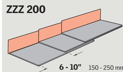
**ENGLISH:** For exposures between 6" (150 mm) and 10" (250 mm), use VELUX step flashing kit ZZZ 200 to replace the standard step flashing pieces and obtain adequate overlap.
