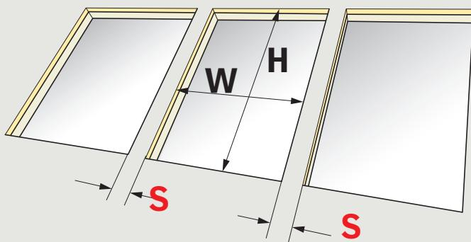
**ENGLISH:** Prepare rough openings with spacings and dimensions as shown. Use spacing **S** that corresponds to a (nominal frame spacing). Frame spacing **a** is specified on the EKL ---8 gutter.
