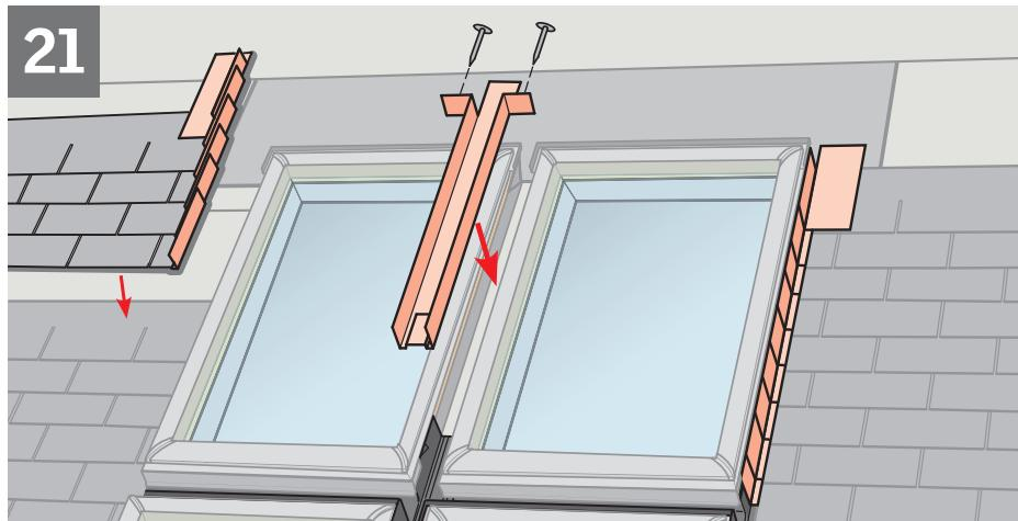
**ENGLISH:** Install roofing material (see **9**), step flashing pieces and gutter.
