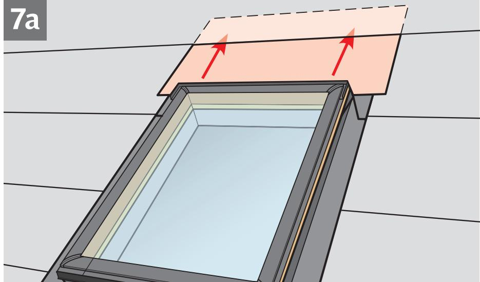
**ENGLISH:** To allow for proper drainage, interweave VELUX adhesive skylight underlayment as shown in **7a** for new construction applications. For retrofit applications, interweave VELUX adhesive skylight underlayment as shown in **7b**.
