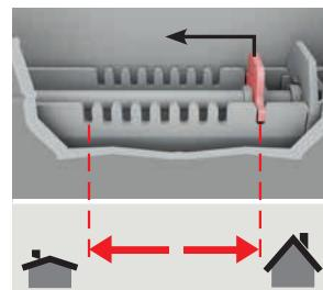
**ENGLISH:** The sash should be able to remain open in any position; otherwise, springs must be adjusted as shown.
