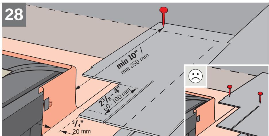
**ENGLISH:** Observe distance to roofing material. Do not nail through the saddle flashing when attaching the roofing material.
