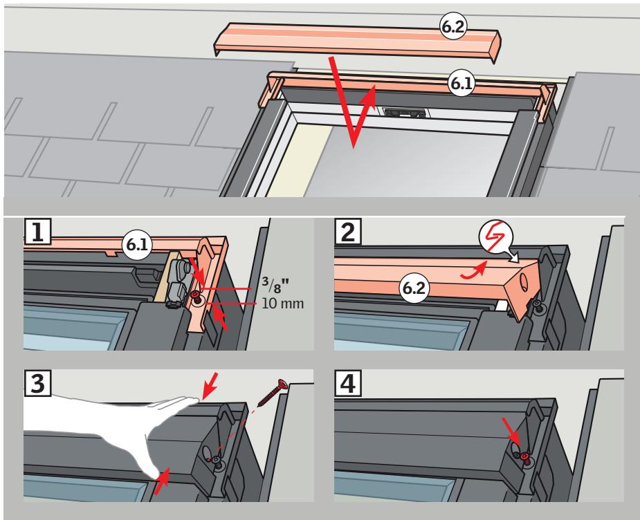
**ENGLISH:** Install and secure the two top frame cladding parts as shown. Make sure the cladding parts engage correctly (1, 2, 3, 4).
