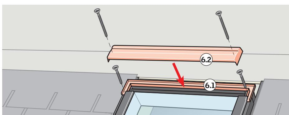
**ENGLISH:** Install and secure the two top frame cladding parts as shown.
