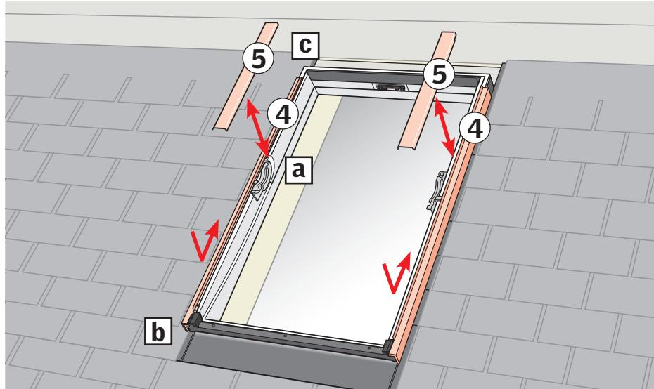
**ENGLISH:** Remove cladding parts shown (a). Install and engage cladding parts as shown (b, c). Long windows: Bend over frame flaps to secure.
