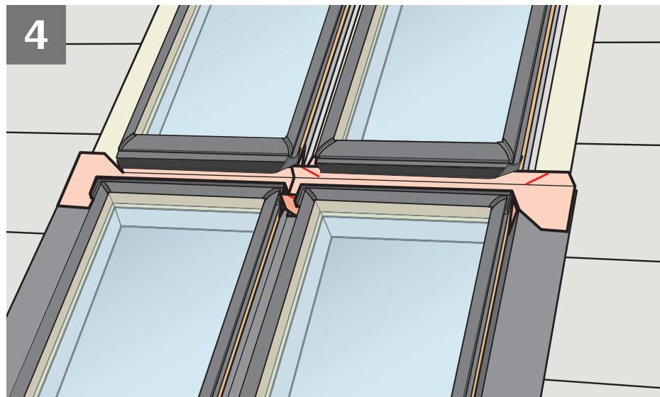
**ENGLISH:** Wrap top and bottom frames and the corners of the skylight/roof window with VELUX adhesive skylight underlayment and create proper water-shedding lap.
