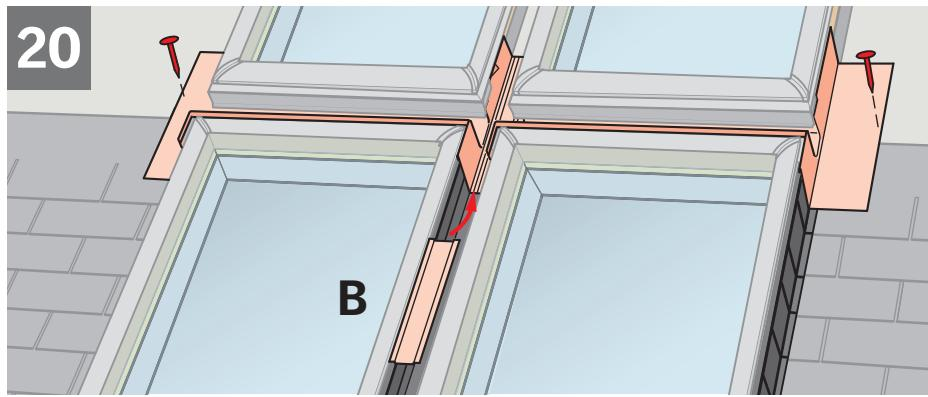
**ENGLISH:** Interlock middle flashing sections using the long 16" (405 mm) slide strip (**B**) and flatten with hammer to lock. Attach middle sections at the sides **a**.
