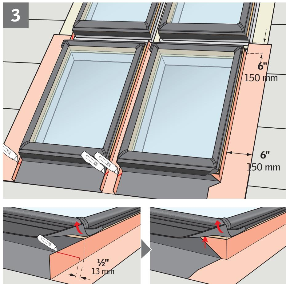
**ENGLISH:** Wrap the side frames and corners of the skylight/roof window with VELUX adhesive skylight underlayment and create water-shedding laps over roofing underlayment.
