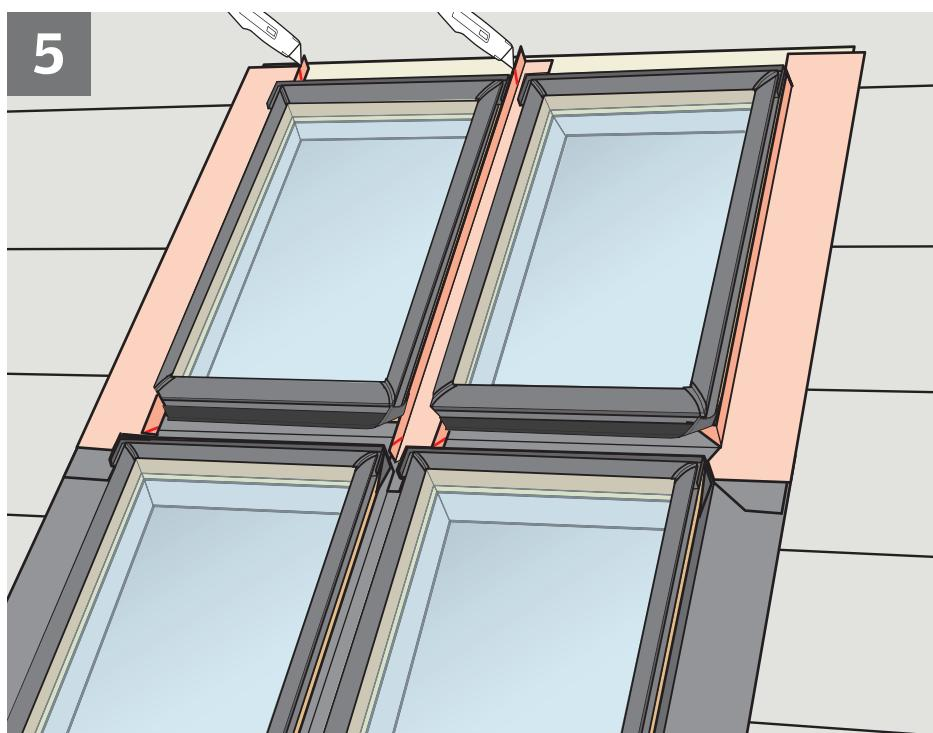
**ENGLISH:** Wrap the side frames and corners of the skylight/roof window with VELUX adhesive skylight underlayment and create water-shedding laps over roofing underlayment.
