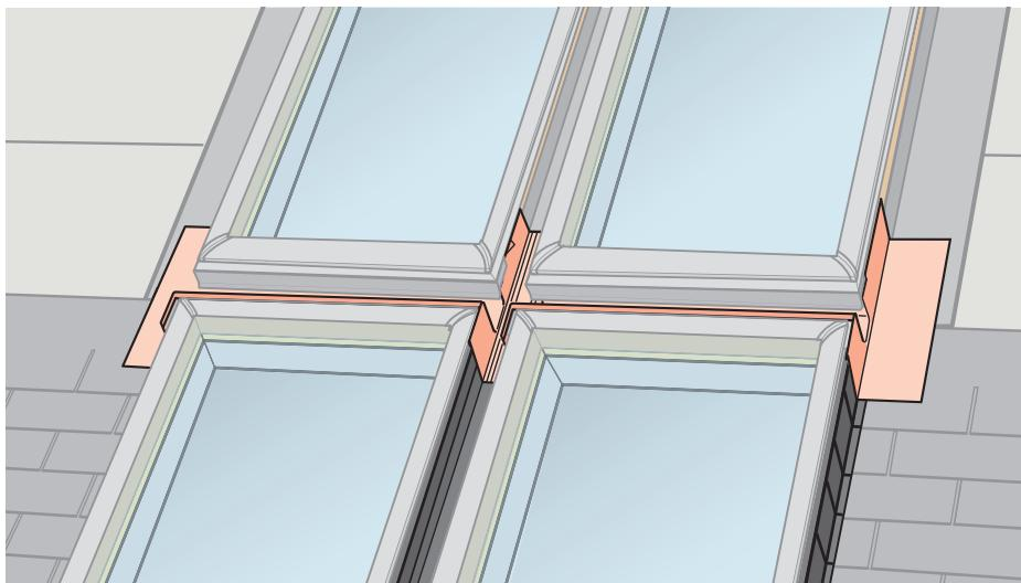
**ENGLISH:** Install middle flashing sections. Determine use of extension piece: use it if the middle sections are lifted up by the underlying roofing material and remove it if the middle sections fit tightly over the skylights/roof windows.
