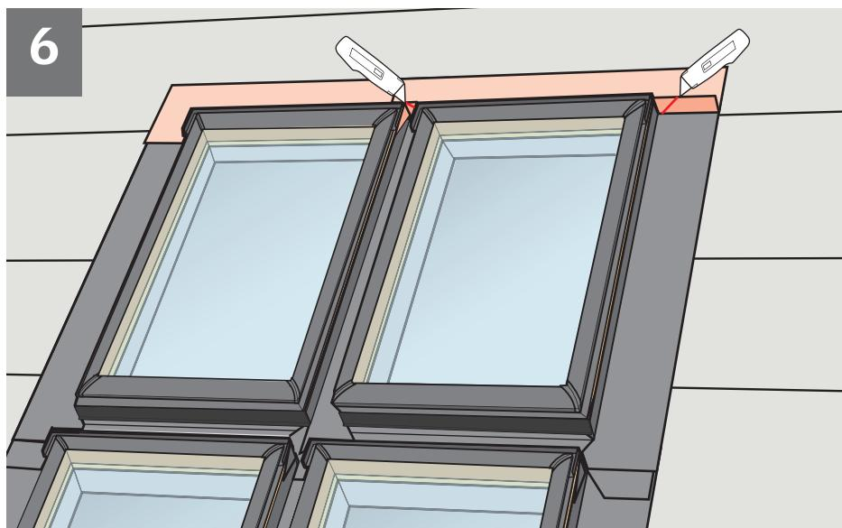
**ENGLISH:** Wrap the top frame and corners of the skylight/roof window with VELUX adhesive skylight underlayment and create proper water-shedding lap.
