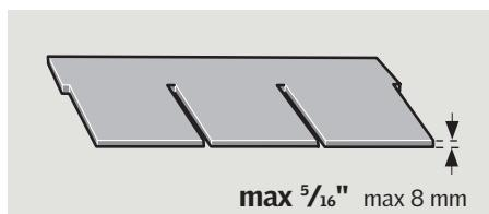
**ENGLISH:** EKL is designed for thin roofing materials (max thickness 5/16" (8 mm)).
