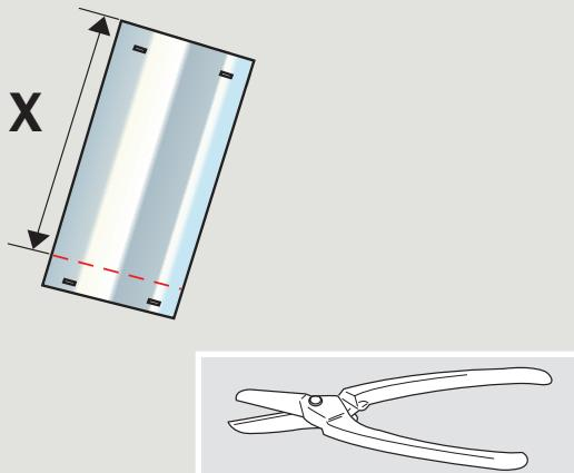
**ENGLISH:** With one rigid tunnel section, cut the section to length (**A**).
