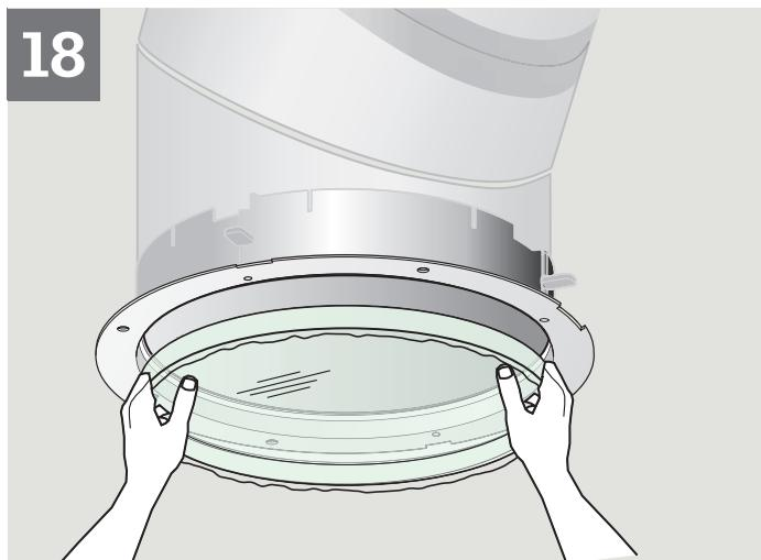
**ENGLISH:** Install the diffuser with the frosted side facing down.
