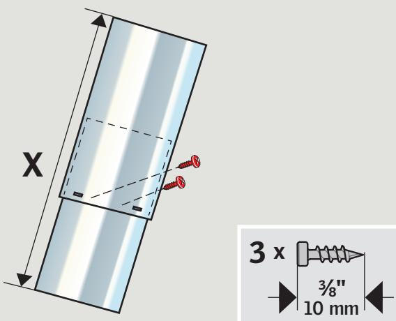
**ENGLISH:** With two tunnel sections, reduce the length of the tunnel assembly by increasing overlap. Secure the joint with three of the  $\frac{3}{8}$ " (10 mm) screws (**B**).
