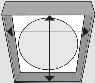
**ENGLISH:** To make the flashing fit properly on the curb, the curb and roofing material dimensions must be less than the flashing clearance, ie  $20\frac{7}{8}'' \times 20\frac{7}{8}''$  (530 mm x 530 mm).
