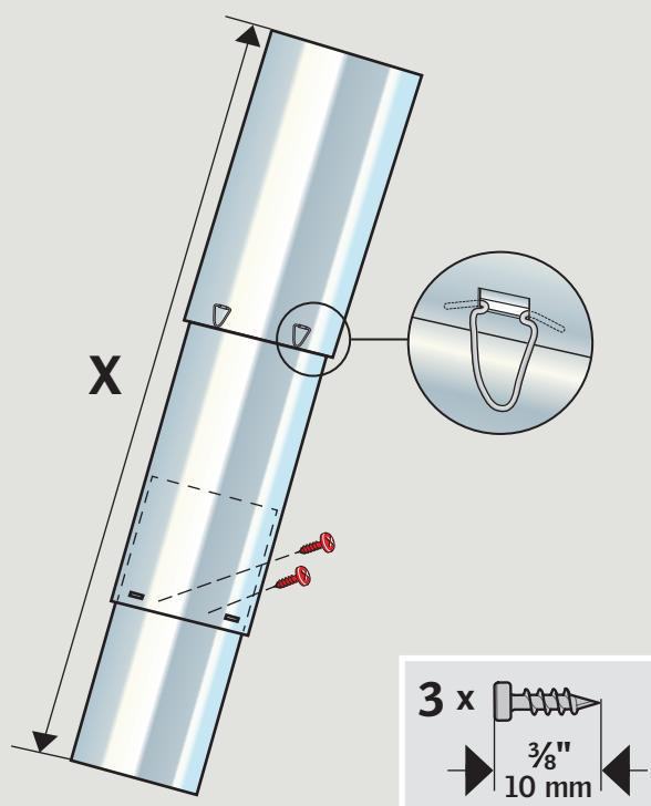
**ENGLISH:** With more tunnel sections, assemble the upper sections with the tunnel clips provided and reduce the length of the tunnel assembly by increasing overlap at the bottom. Secure the joint with three of the  $\frac{3}{8}$ " (10 mm) screws.
