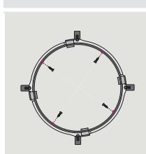
**ENGLISH:** Secure tunnel assembly to ceiling ring with four of the  $\frac{3}{8}$ " (10 mm) screws provided.
