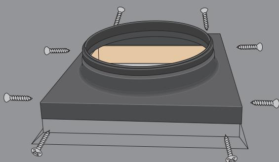
**ENGLISH:** Install and secure the flashing with  $1\frac{3}{4}''$  (45 mm) screws provided.
