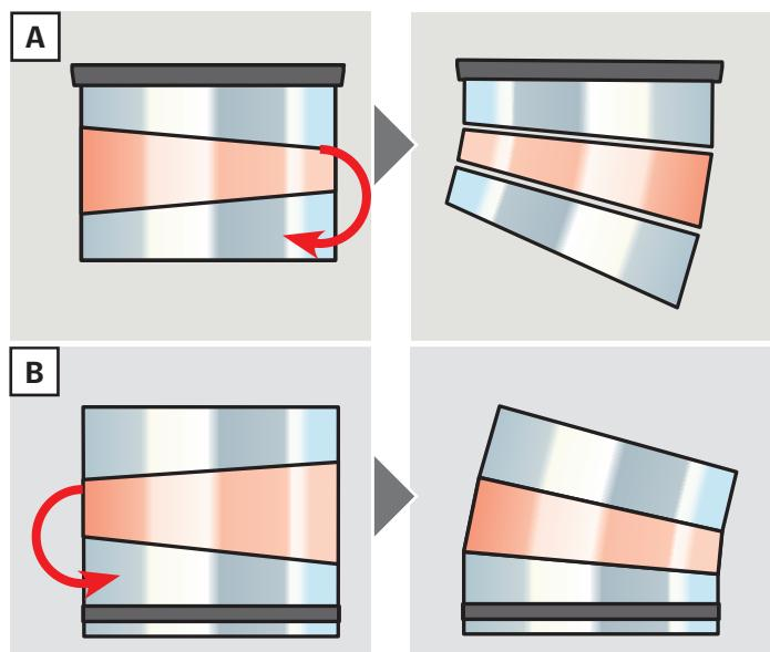
**ENGLISH:** Adjust the angle of both elbows so that they point directly against each other **A, B**. Elbows can be damaged if excess force is applied.
