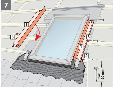
1 Slide side flashing sections to interlock with
