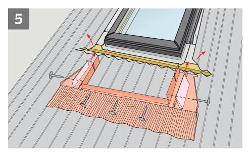
Cut foam down to level of underside of metal roofing to ensure that roofing lies flat.
