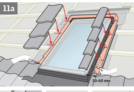
Trim foam gasket and flatten upstands on side sections as necessary. Make a slit above each tile to allow foam gasket to seal against underside of tile. Maintain distance to frame as shown; cut tiles if necessary. To make tile lie correctly it may be necessary to remove neck on tile and flatten the returned edge around the battens.
