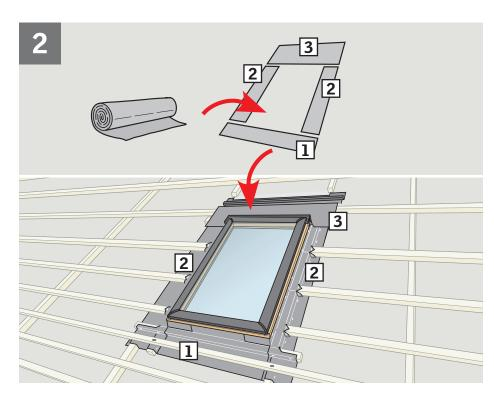
If roofing underlay is used (provided by installer): Dress roofing underlay up around all four sides of the frame. Roof with counter battens shown for illustration purpose.
