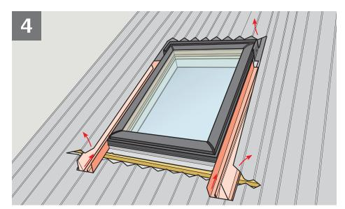
Fit the side flashing sections under the existing metal roof and the top flashing section.
