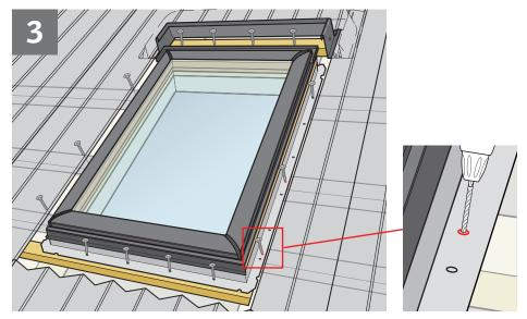
Check level at bottom of frame and fix the angle brackets on the skylight to the rafters.
