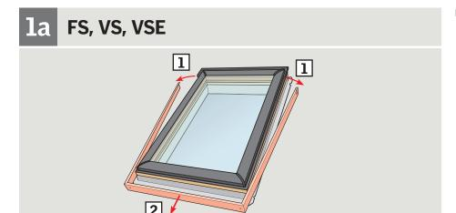
For proper installation, remove cladding as shown
