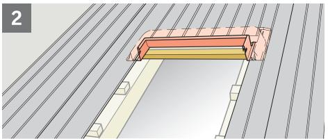
If it top flashing section under the existing metal roof before laying the skylight in position. Take care to maintain 30-60 mm distance from sides of frame to metal roof, 100 mm below and 60-150 mm above skylight.
