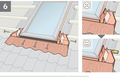
Position bottom flashing section as shown and install battens to support joints with side flashing sections if necessary.
